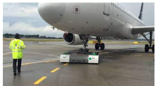
Figure 5 Ground crews remotely controlled the aircraft tug to push back the A320 at Changi Airport [17].
