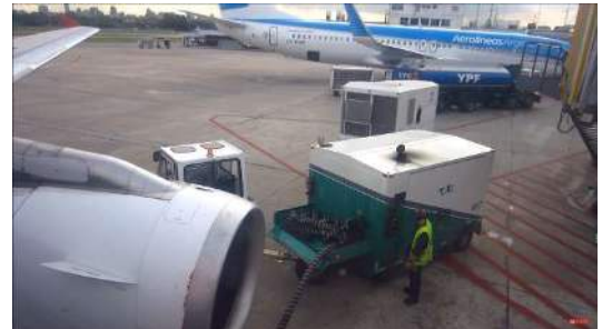
Figure 4 AIRSTART of IAE engine with Air Starter Unit (ASU) - LATAM Airbus A320 [16]
