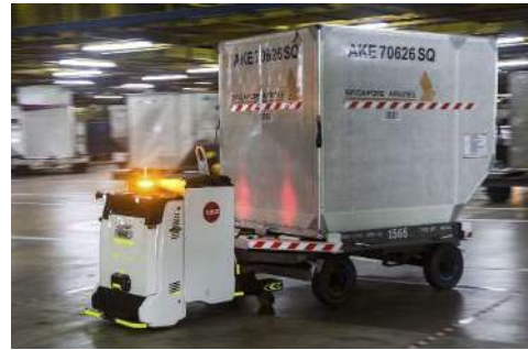
Figure 13 Autonomous Container Trailer [27]
