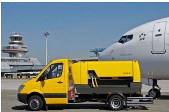
Figure 19 Ground Power Unit Vehicles [45]
