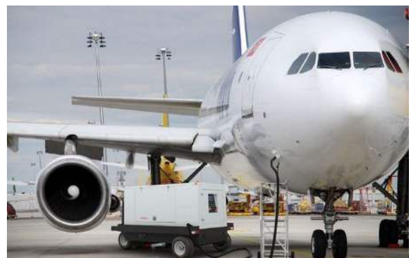
Figure 7 400Hz Ground Power Units powering an aircraft [18]
